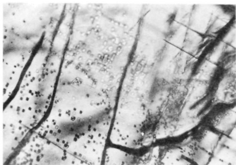
Figure 7. Etch pits on the (010) face of 2 after partial dissolution in presence of 1a .
